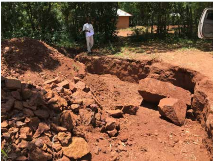
FIGURE 9: TYPICAL RED-COLOURED FERRASOL SOIL IN WHICH A VERY HARD HORIZON OF LATERITE / FERRICRETE HAS DEVELOPED. THESE SECONDARY ROCKS ARE LOCALLY MINED AND CUT INTO SUITABLE SIZES WITH SUITABLE SURFACES (STONE DRESSING) AND USED TO CONSTRUCT FOUNDATIONS OF HOUSES. PHOTO TAKEN AT LAT: 0.3163 / LON: 34.0632 / 1162 M
