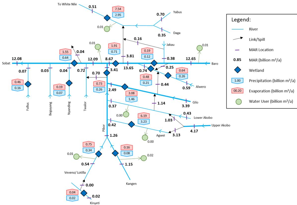
Figure 11-45: Water balance of the Baro-Akobo-Sobat sub-basin
