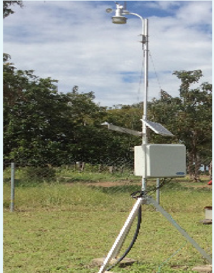
AN AUTOMATIC WEATHER STATION INSTALLED BY NELSAP
