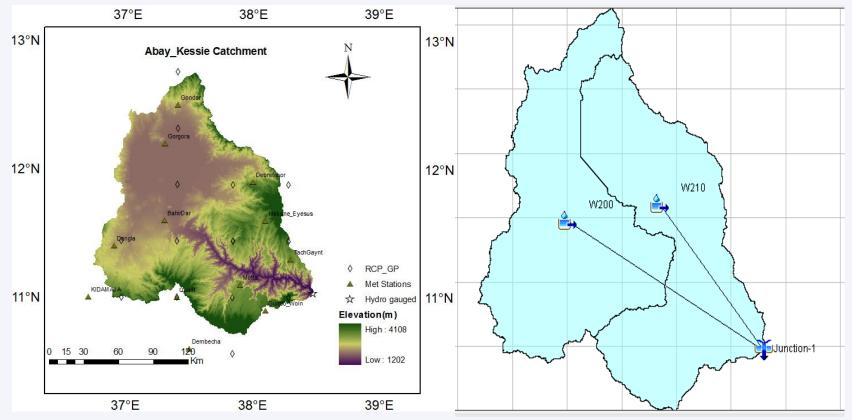
HEC-HMS4.2 hydrologic modelling basin model physical watershed map for Kessie catchment during calibration.
