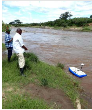
Using Acoustic Doppler Current Profiler for the river hydraulic profiling.
