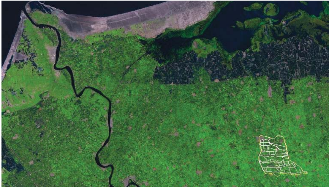
Detailed False Color Composite of a Landsat Thematic Mapper image acquired on 25 June 2008. In this case green represents a high near-infrared reflectance, being a characteristic for vigorous crop growth. The more green, the better the agricultural production. The Western branch of the river Nile (Rosiette Branch) is visible. The purple color represents urban areas (light purple) or sand dunes and beach (bright purple). The black color are wetlands and fishponds. The inset with the yellow boundaries displayed is the W10 area, being a pilot zone of the IIIMP project. The W10 tertiary irrigation system
