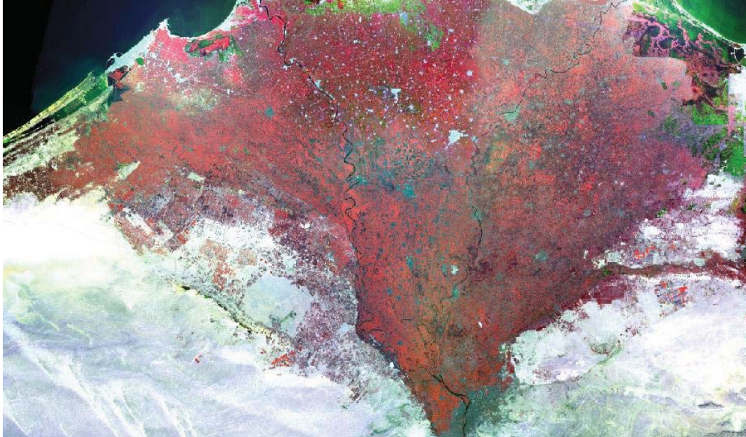
False Colour Composite (FCC) images based on Landsat Thematic Mapper measurements. This FCC images is compiled from different individual Landsat images for the purpose of covering the entire Nile Delta. Red colours express a high near-infrared reflectance, being a characteristic for vigorous crop growth. The more red, the better the agricultural production. The white areas are bright desert sandy soils.
