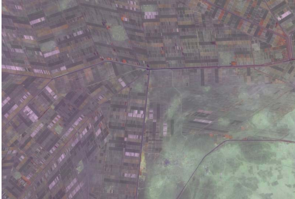
Landsat image of the central part of the Gezira scheme. Fields with a red color are cropped. The dark colored fields are bare. The fields with white color are vegetables with specific mulch treatments
