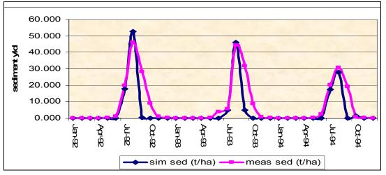
Figure 5.12 Comparison of observed monthly sediment with simulated monthly sediment at Gilgel Abbay
