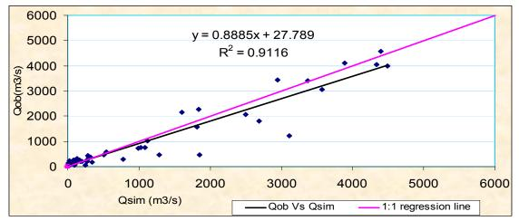
Figure 5.6Regression analysis line and 1: 1 fit line of measured versus simulated flow at Kessie
