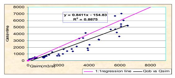
Figure 5.7Regression analysis line and 1: 1 fit line of measured versus simulated flow at Border
