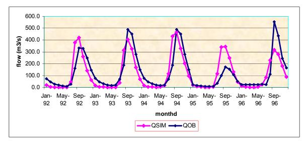
Figure 5.2Comparison of simulated Vs. measured stream flow at Bahirdar outlet for model calibration
