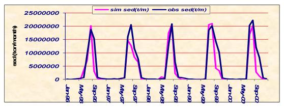
Figure 5.20Comparison of observed monthly sediment carried Vs simulated monthly sediment carried during validation at Kessie
