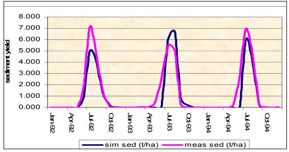
Figure 5.13 Comparison of observed monthly sediment with simulated monthly sediment near Kessie
