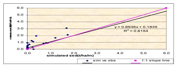
Figure 5.17Regression analysis and 1: 1 fit line of measured versus simulated sediment yield at Kessie
