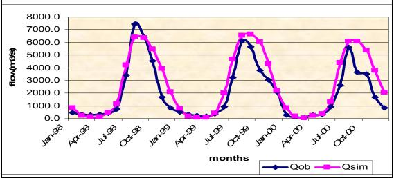
Figure 5.10Graphical comparison of measured Vs. validation Simulated flow at Border outlet
