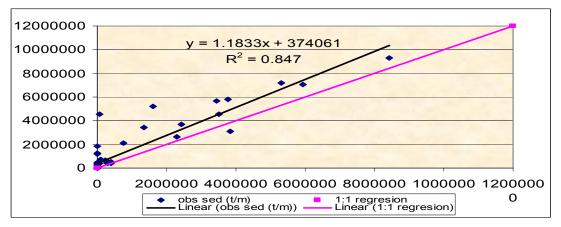
Figure 5.19Regression analysis line and 1:1 fit line of monthly measured sediment load versus simulated sediment load transported Gilgel Abbay
