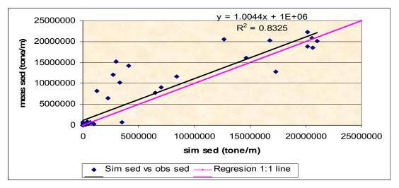
Figure 5.21Regression analysis and 1:1 fit line of monthly measured sediment load versus simulated sediment load transported at Kessie
