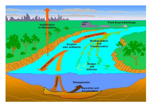
Figure 2.6 : In stream processes modeled by SWAT
