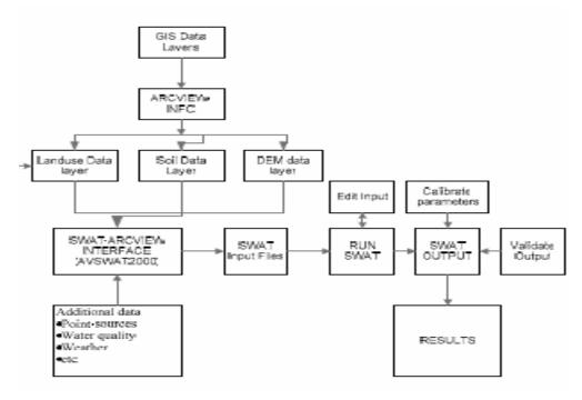
Figure 4.1The general layout of Simulation diagram of SWAT model
