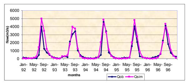
Figure 5.3comparison of simulated Vs. measured stream flow at Kessie outlet for model calibration
