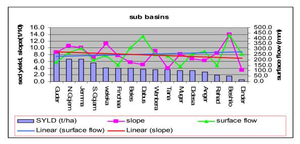
Figure 5.23 The graphical comparison of the effect of surface runoff and slope steepness on sediment yielding
