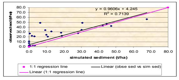
Figure 5.15Regression analysis and 1:1 fit line of measured versus simulated sediment yield at Gilgel Abbay
