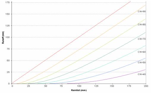
Figure 2.5: Relationship of runoff to rainfall in SCS curve number method
