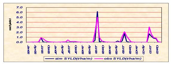
Figure 5.16Comparison of observed monthly sediment yield with simulated monthly sediment yield during validation at Kessie
