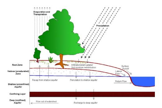
Figure 2.3 Schematic representation of the hydrologic cycle.
