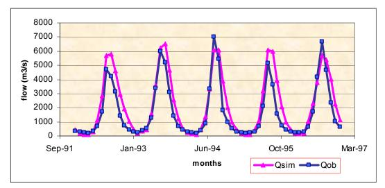
Figure 5.4comparison of simulated Vs. measured stream flow at Border outlet for model calibration
