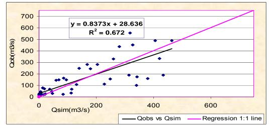
Figure 5.5Regression analysis line and 1: 1 fit line of measured versus simulated flow at Bahirdar
