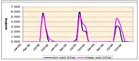
Figure 5.11 Comparison of observed monthly sediment with simulated monthly sediment at Addis Zemen
