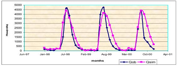
Figure 5.9Graphical comparison of measured Vs. validation Simulated flow at Kessie outlet
