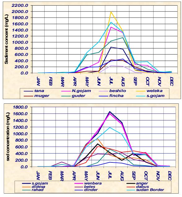
Figure 5.25a & b Comparisons of sediment concentration at the outlet of each sub basins
