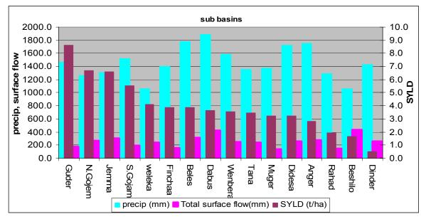
Figure 5.24 Graphical relation of sediment yield, precipitation and surface run off
