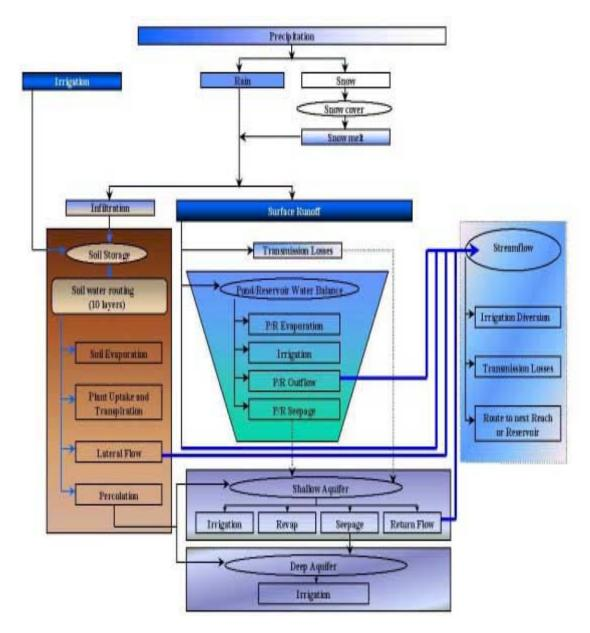
Figure 2.2 over view of SWAT hydrologic component (Arnold et.al, 1998)
