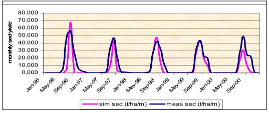
Figure 5.14Comparison of observed monthly sediment yield with simulated monthly sediment yield during validation at Gilgel Abbay
