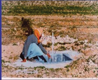
Run off measurement after rain-storm
