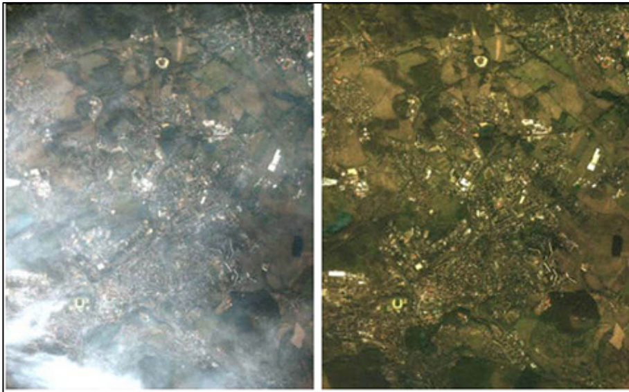
Figure 3 Illustration of the atmospheric correction using Sen2Cor algorithm. (Left) before atmospheric correction, (right) after successful atmospheric correction
