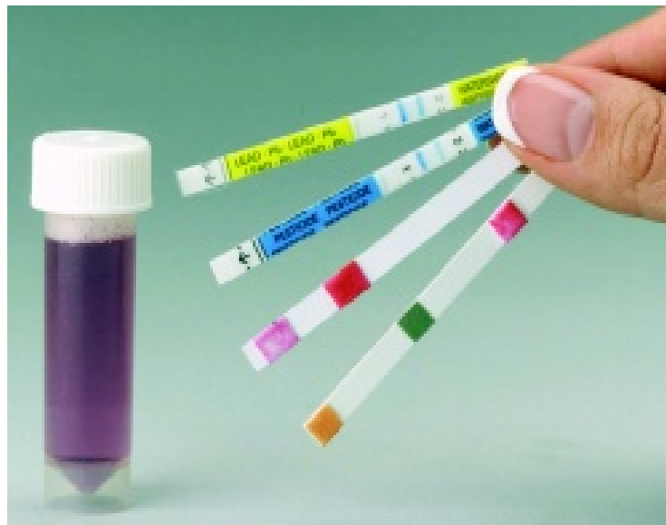
Fig.(1) Water quality test kit (H2OKIT)
