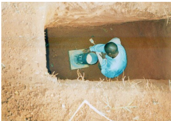
In-situ density test being conducted in one of the test pits
