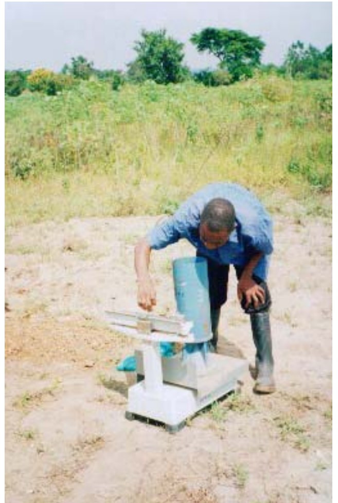
Weight measurements for in-situ density tests
