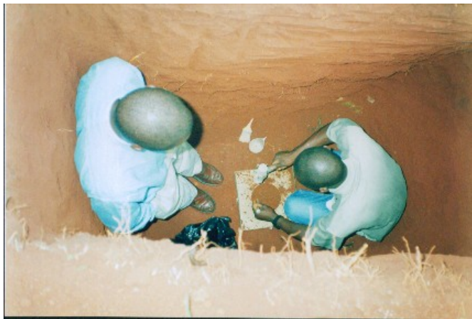
In-situ density test being conducted in one of the test pits
