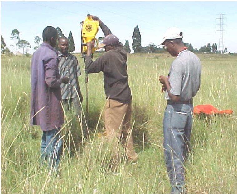
Plate 2 Dynamic sounding test at different depth
