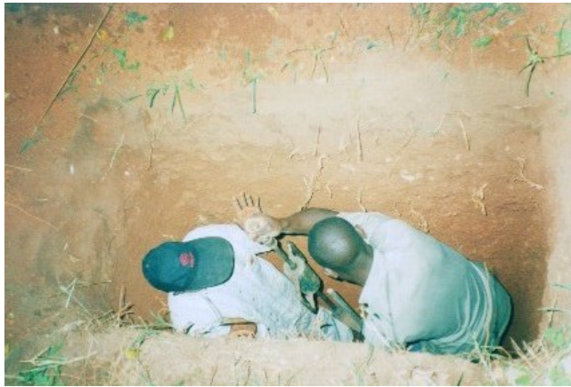
Dynamic Cone Penetration (DCP) test being carried out in one of the test pits
