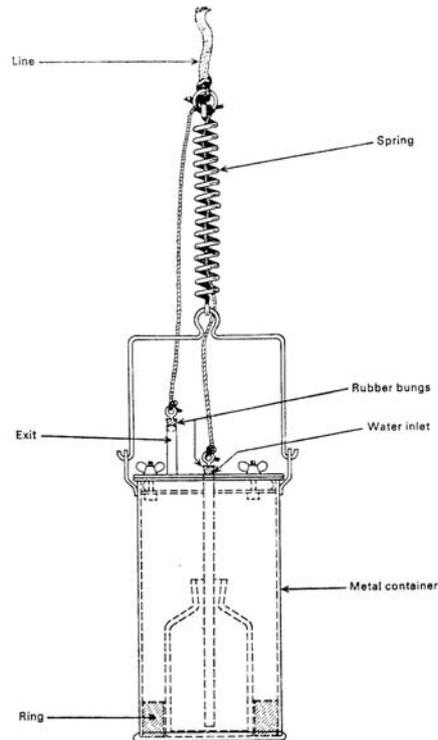
When the sampler is at the require depth, a sharp tug on the line will release the inlet and outlet bungs to allow the water to be sampled.
