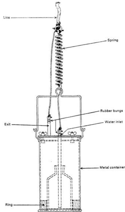
When the sampler is at the require depth, a sharp tug on the line will release the inlet and outlet bungs to allow the water to be sampled.
