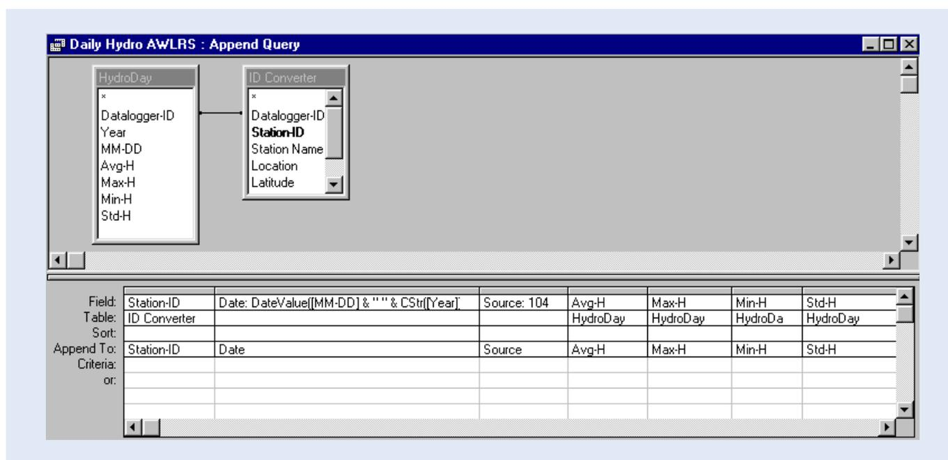
The query employs two tables: ID-Converter and an auxiliary MS Access table, in this case HydroDay. The tables are linked through the Datalogger-ID field.
