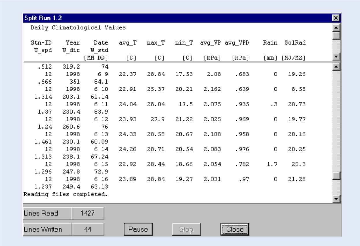
For every day the Met Station has been operational, the following information is generated: station-ID, year and date; average, maximum and minimum daily air temperature; average vapor pressure and vapor pressure deficit; total daily rainfall and solar radiation; average daily wind speed and direction, as well as standard deviation of the wind direction.
