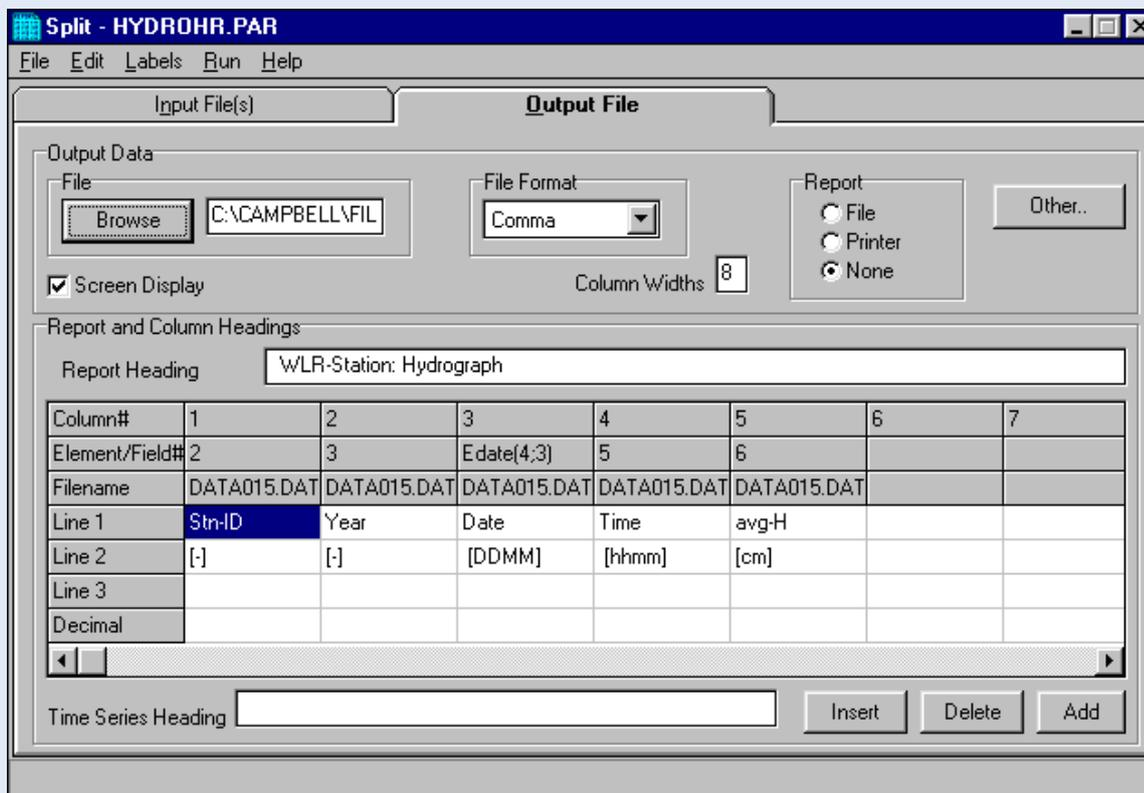
Step C6: Select location for, and give a name to, the resulting Output file. To this end click "Browse" in the Output Data box. Navigate to the desired folder on the hard drive and type in an output file name according to the following convention:
