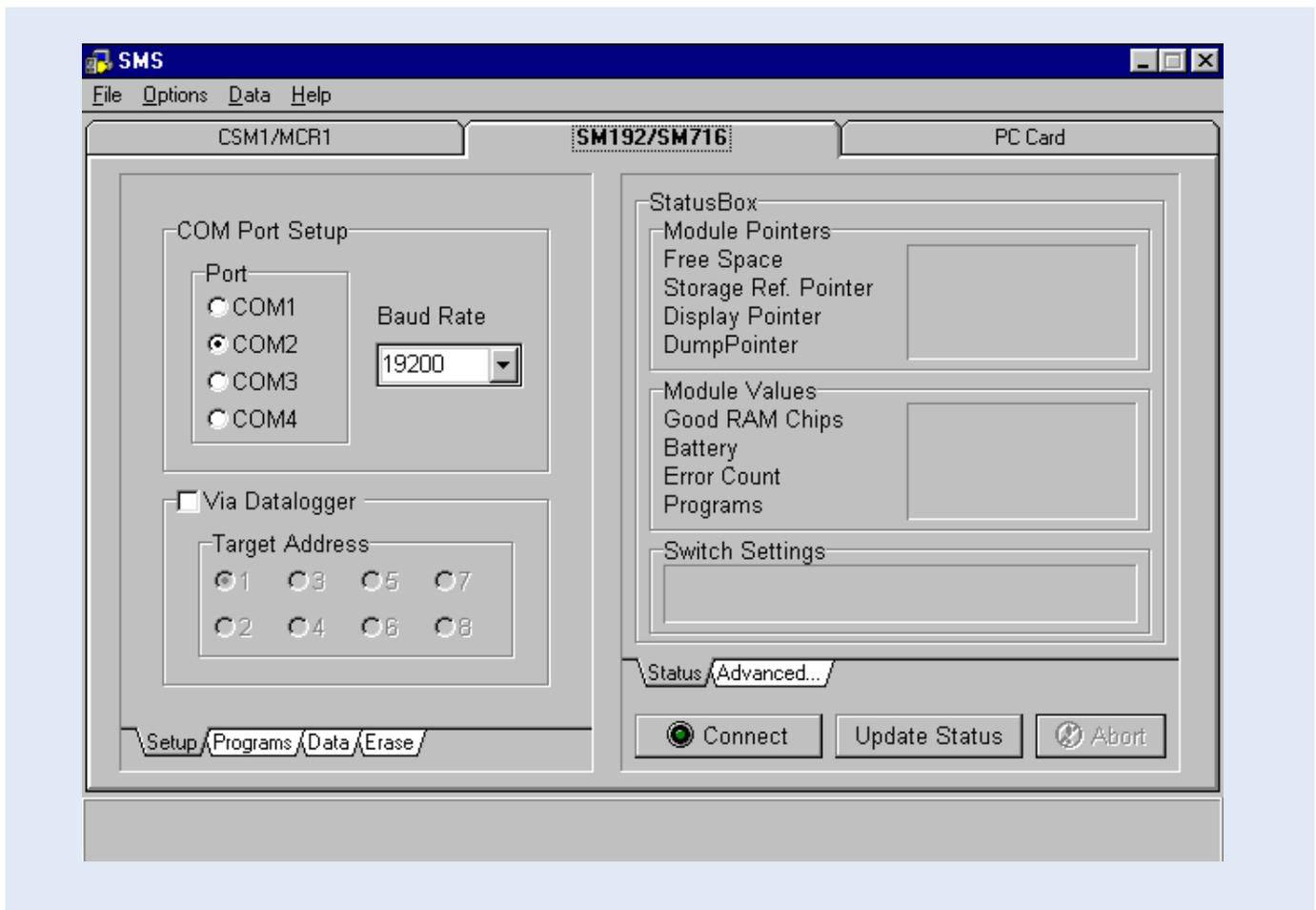
Step A7: Select the COM Port settings corresponding to the serial port used by the "9 to 25" computer cable connecting the SC532 Interface (see paragraph 3.1). In most cases this will be either COM1 or COM2.
