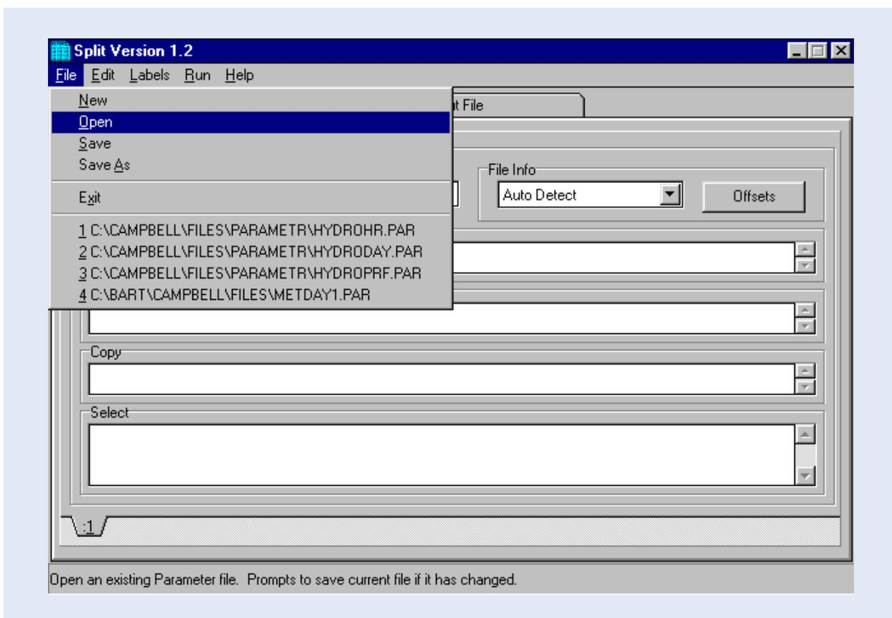
Step C3: Navigate to the location on hard drive which contains the parameter files. This is "C:\CAMPBELL\FILES\PARAMETR" if the Recommended Directory Structure is used. Highlight the file "hydrohr.par", as shown on the window below. Click OK.
