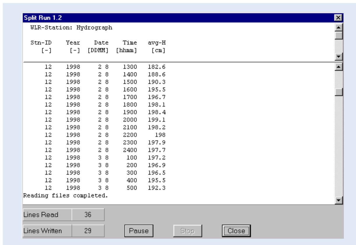
For every hour, the following information is generated: Station-ID, Year, Date, Time and Average 1-Hour Water Level in cm. The first four items of this list uniquely identify each output array.
