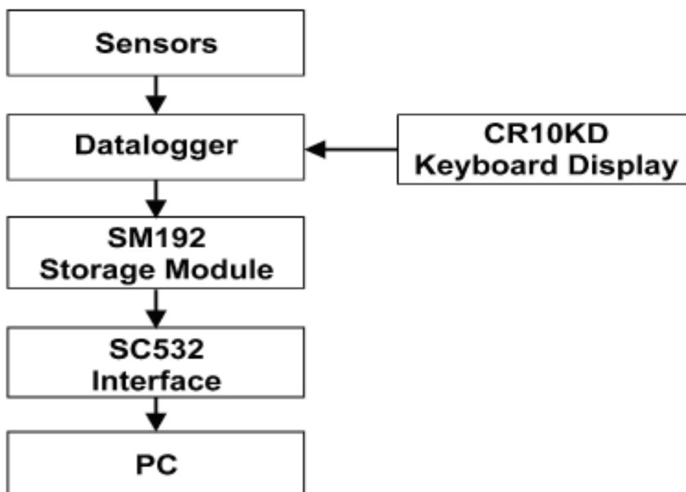
Figure 1: Hardware components involved in data acquisition process.
