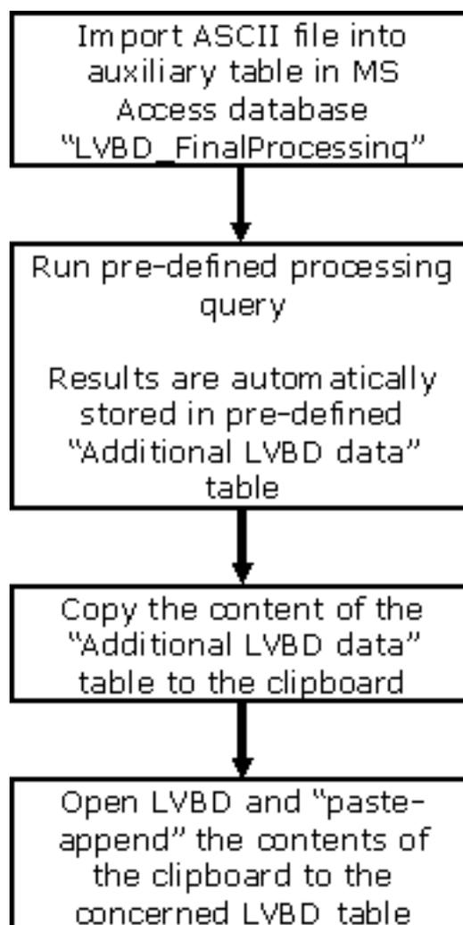
Figure 5: Final data processing steps in MS Access.
