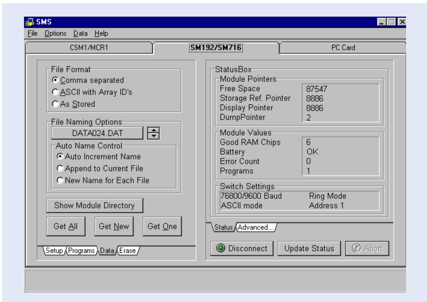
Step B4: Mark the "Auto Increment Name" option in the Auto Name Control select box. Each retrieved data file will get a name according to the format "DATAXXX.DAT" in which XXX is a number which automatically increments when a new file is down loaded.
