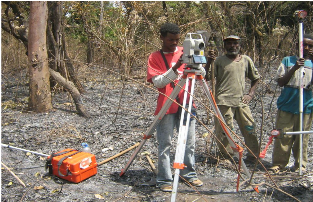
Setting of surveying equipment to take readings of the canal route topography
