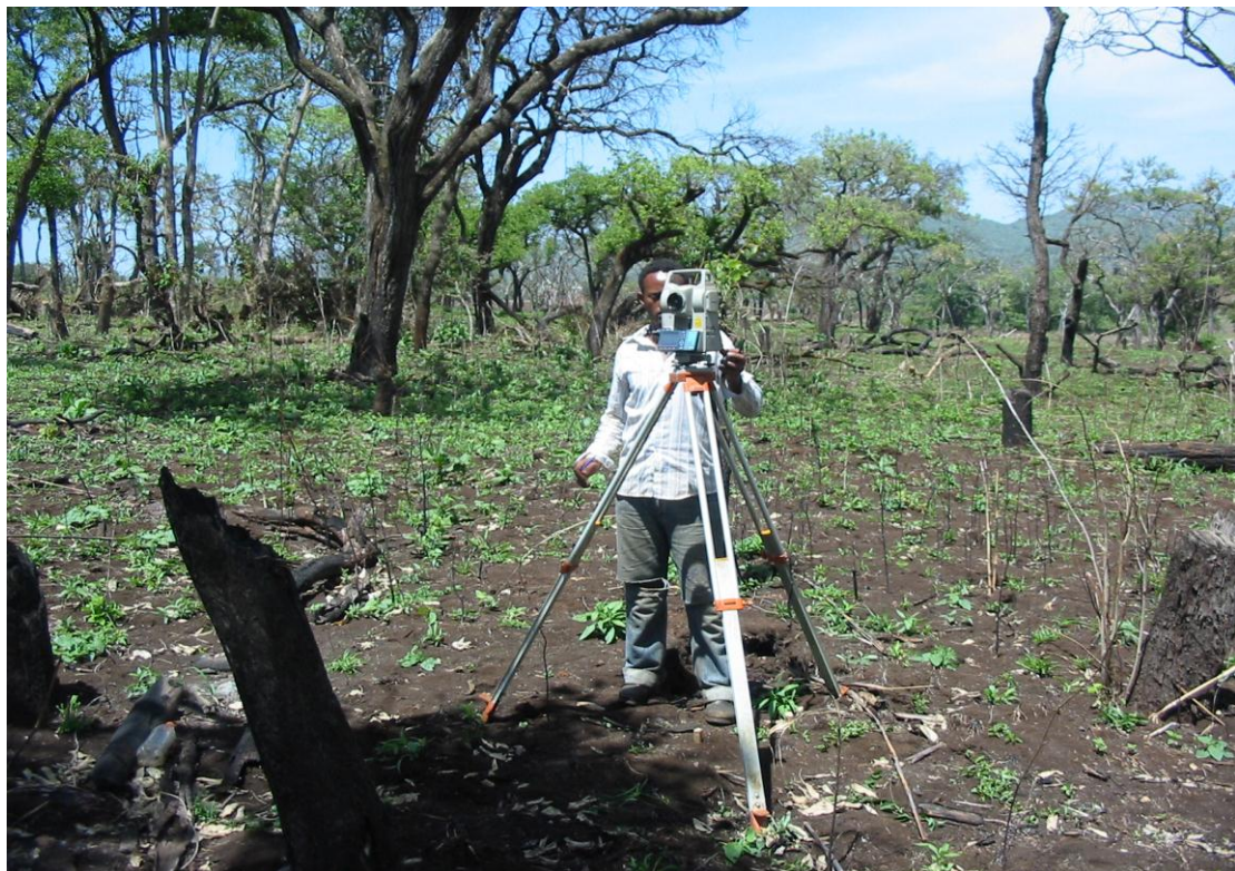
Total station used to survey the command area
