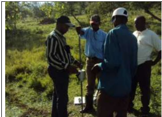
Figure 10: Light Dynamic Cone Penetrometer tests used in Uganda
