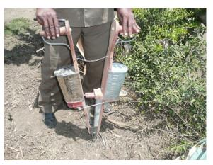
Figure 7.7 (a). Sketch of a hand-jab planter with seed and fertilizer hoppers
