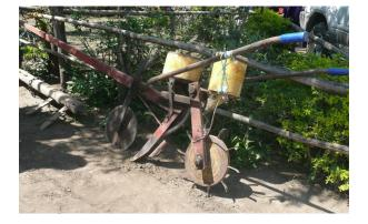
Figure 7.8 (a) Tined openers for animal-drawn no-till planters (source: Ribeiro et al, hopper (photo by Bancy Mati) 2006)
