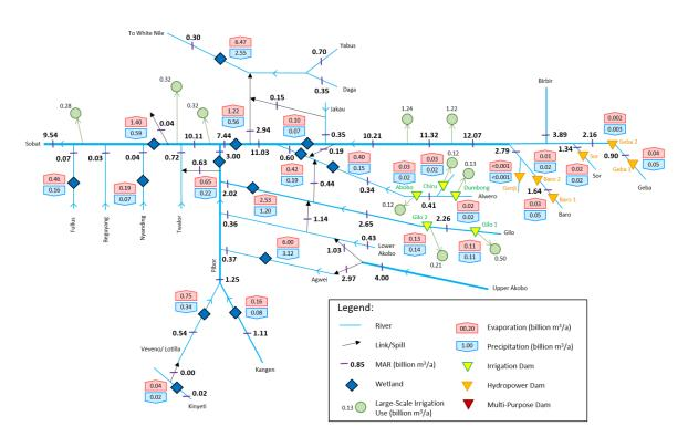
Figure 7-2: Water balance schematic of Scenario 1
