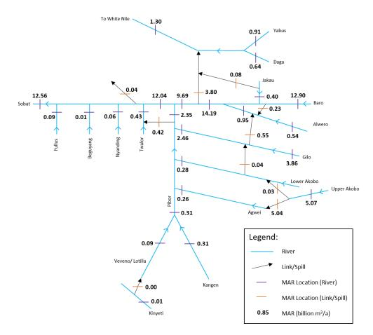
Figure 2-2: Water balance schematic under baseline conditions
