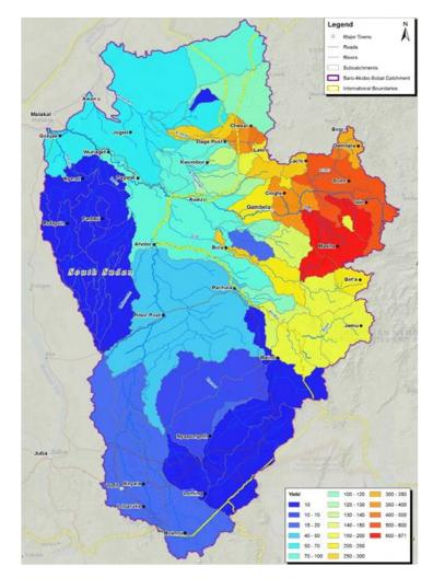
Figure 11-5: Cumulative sediment yield in the basin in t/km2/a
