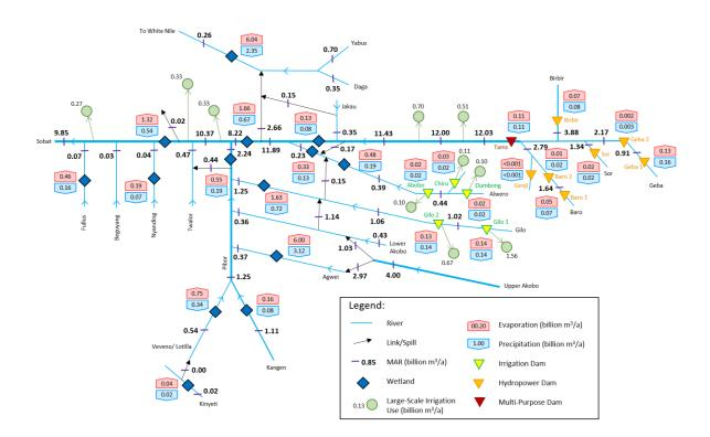
Figure 7-5: Water balance schematic of Scenario 3b
