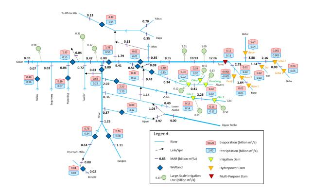
Figure 7-3: Water balance schematic of Scenario 2
