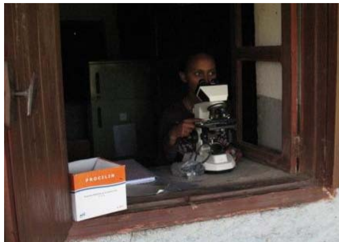
Figure 7-6: Addis Betekristian Health Centre (Fogera Woreda): microscopic observations using sunlight for illumination due to lack of electricity
