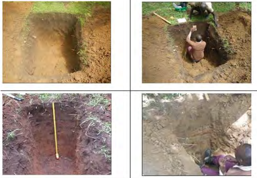
Plate 1: Soil Characterization Test Pits
