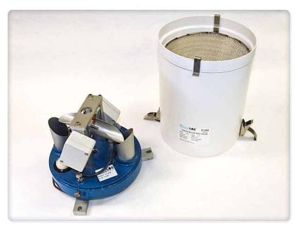
Figure 5-3: Tipping Bucket (WaterLOG YSI incorporated, used by permission)
