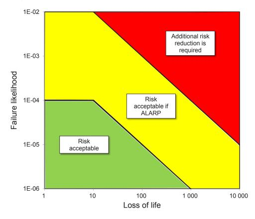
Figure 2: Risk levels for Dam Safety using loss of life societal consequences
